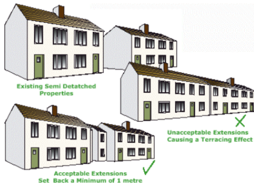
Fig C: illustration of how setting back by as little as 1 metre can reduce the impact of the extensions on the street scene by avoiding the creation of a terrace.
